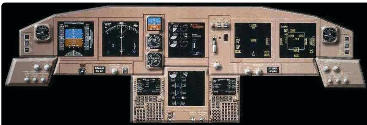
Figure 1-5. Electronic Displays are driven by Symbol Generators.
