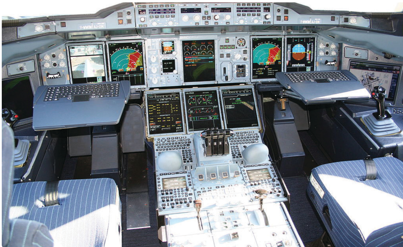
Figure 1-2. Airbus A380 EIS with 8 Large LCD Displays.
