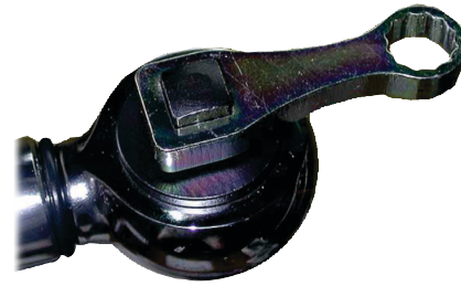
Figure 3-16. A typical torque wrench extension in the straight position.
