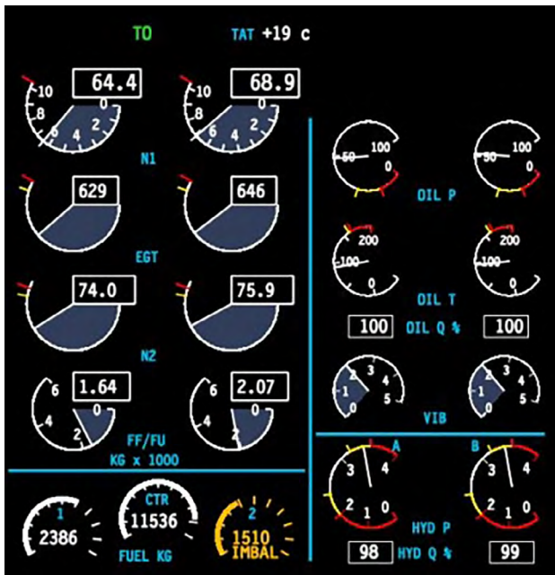
Figure 1-9. EICAS engine display format.
