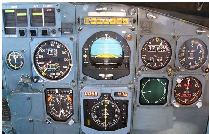
Figure 1-3. Equivalent electromechanical flight and navigation instruments on the left.
