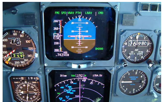
Figure 1-3. Equivalent electromechanical flight and navigation instruments on the left.
