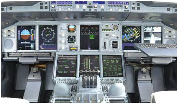
Figure 1-2. Airbus A380 EIS with 8 Large LCD Displays.
