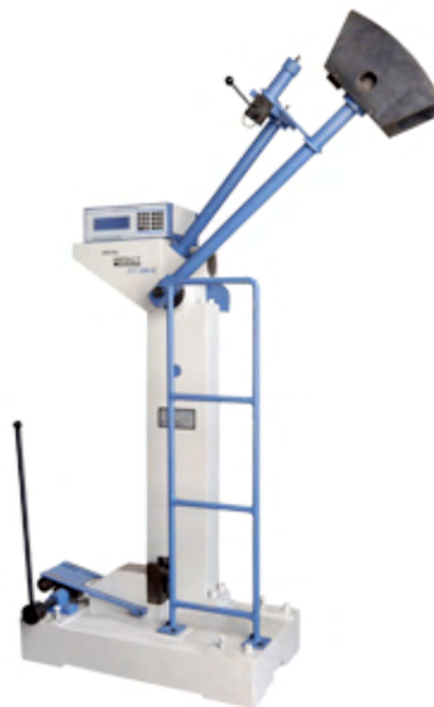
Figure 1-10. An IZOD impact test machine.
