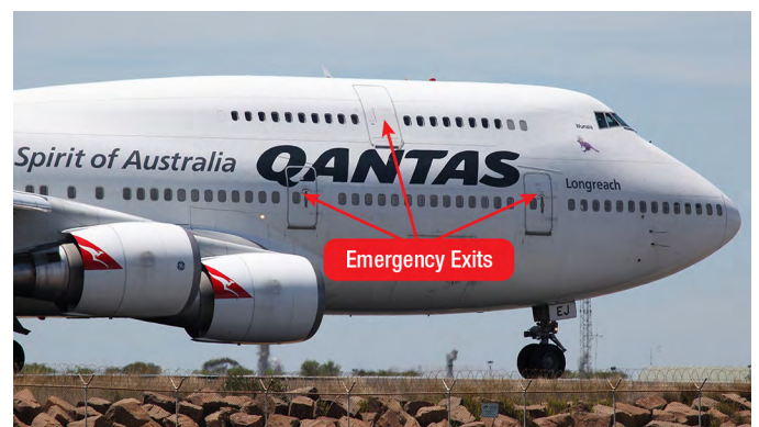
Figure 5-12. Required external emergency exit markings.
