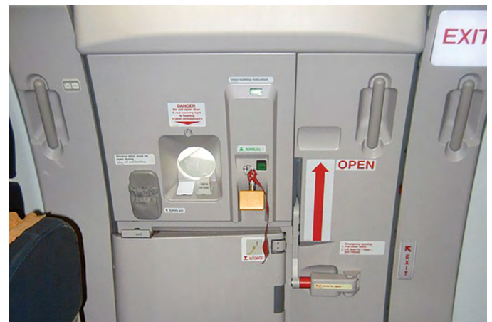
Figure 5-11. Required emergency exit markings.
