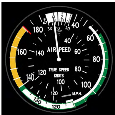
Figure 5-10. An airspeed indicator includes colored markings around its perimeter, highlighting important restrictions for which the pilot must be aware.
