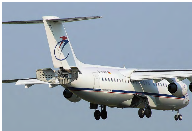
Figure 1-22. The BAe146 speed brake system can be deployed both in flight and after touchdown.
