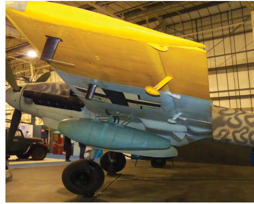
Figure 1-30. An aileron mass balance.
