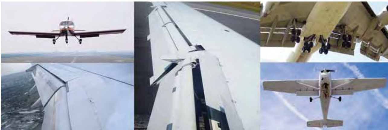
Figure 1-16. Flap extension on large and small aircraft.
