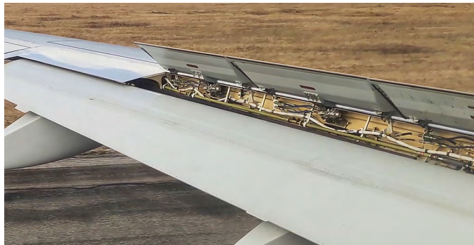
Figure 1-21. Spoilers fully deployed as speed brakes on an Embraer 190.
