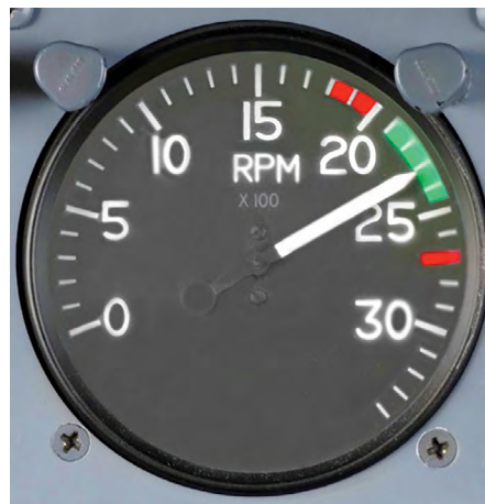
Figure 1-17. Red arc from 1 800 to 2 000 rpm.
